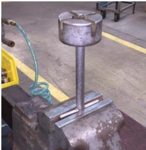
3. From the inlet end of the nozzle heat the stem (web) base with a torch to break down the Loctite. Apply heat in the area where the stem and stem (web) base screw together. Use fireproof gloves and be careful not to burn yourself.
