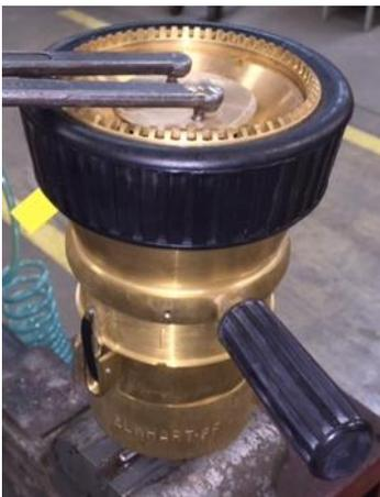
6. Apply 262 (RED) Loctite to the threads on the new stem and thread it into the stem (web) base by hand to make sure the threads are engaged properly and not cross threaded. Screw the stem in until the shoulder bottoms on the stem (web) base and then snug it tight with the wrench. Allow the Loctite to cure for 24 hours before flowing water.
