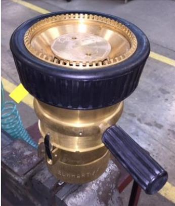
5. Engage the pins of the open face spanner in the stem holes as far as possible and turn the wrench counter-clockwise to unscrew the stem from the stem (web) base.
